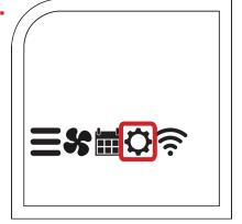
This icon opens the installation settings menu. In this menu, you can adjust advanced preferences for special applications. Select the gear icon, then after IS appears on the screen, select yes to begin the installation settings flow. For more information about the installation settings, please view the "Installation Settings Guide".
