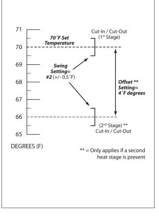
**TEMPERATURE CALIBRATION:** The internal temperature sensor in this thermostat is accurately calibrated at the factory, and in most cases alterations to this setting should not be needed. The Temperature Calibration feature allows you to manually offset the measured temperature by as much as plus or minus 5°F (3°C) degrees from its original value. This feature can be useful to match or synchronize this thermostat to another one or more, if multiple thermostats are used in the same home.
